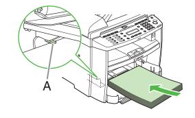
Load the paper into the paper cassette with the print side up. Make sure the paper stack sits below the small fin (A) on the side paper guide.
